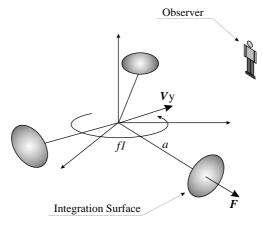
Fig. 13. Scheme of Test 2. A radial compact dipole is described as a small disk with a pressure jump uniformly distributed on its surface. One and three disks at a constant angle from each other are considered, rotating around a vertical axis at the frequency  $f_1$ . The system translates at the velocity  $\mathbf{v}_y$ , whereas the observer is fixed.
