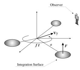
Fig. 20. Scheme of Test 3. An axial compact dipole is described as a small disk with a pressure jump uniformly distributed on its surface. Three and four disks at a constant angle from each other are considered, rotating around a vertical axis at the frequency  $f_1$ . The system translates at the velocity  $\mathbf{v}_{y}$ , whereas the observer is fixed.
